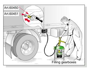
Hand-operated pump for transferring grease: suitable for easy and clean filling of gearboxes, crankcases, manual grease guns etc.
