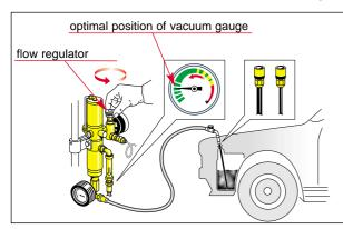
For optimal draining, the pump must function SLOWLY.
