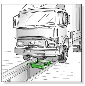
Pit oil drainer, suitable for gravity draining of engine, gearbox and differential oil from all motor vehicles placed on a pit. The tank has an antisplash screen which can also be used as a support for draining the oil filters. The wheel-mounted supports used to handle the tank are adjustable. The 65-litre tank is equipped with a removable side oil conveyor.
