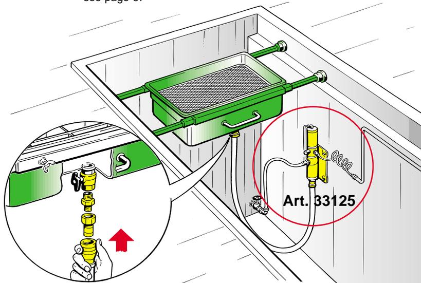
Possibility of applying connections (quick-connector art. 33126-33127) to connect the tank to a pump art. 33125.
