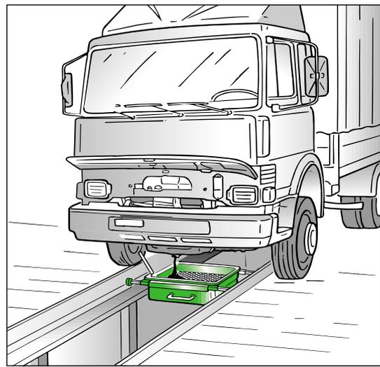
**Pit oil drainer**, suitable for gravity draining of engine, gearbox and differential oil from all motor vehicles placed on a pit. The tank has an antispash screen which can also be used as a support for draining the oil filters. The wheel-mounted supports used to handle the tank are adjustable. The 65-litre tank is equipped with a removable side oil conveyor.
